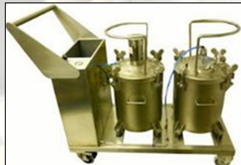
Mobile Cleaning Skid
